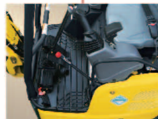
Walk-through operating area
