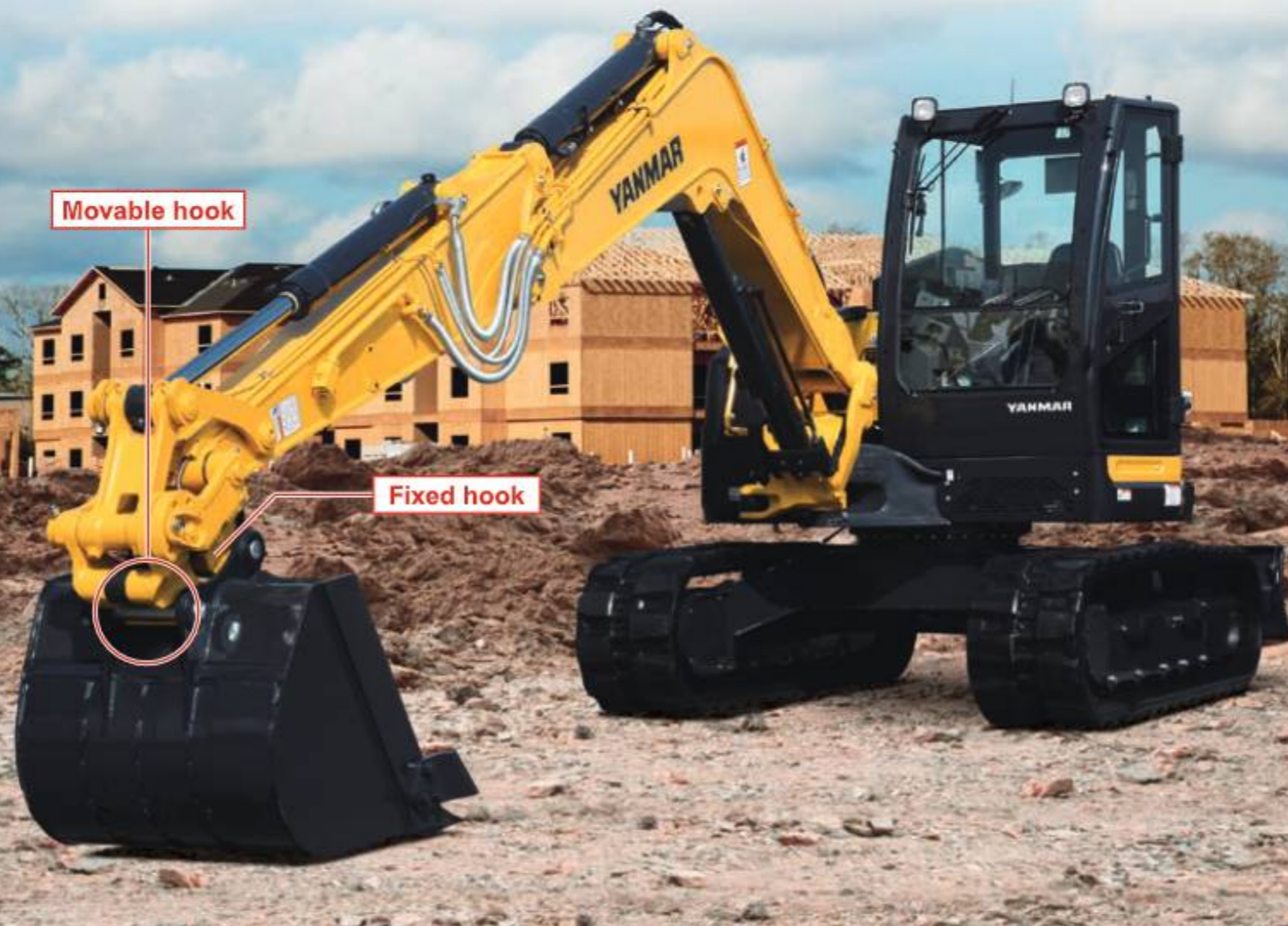
Apply the fixed hook Make the bucket level. Turn the switch to mounting Insert the safety lock pin and fasten.
