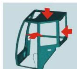
ROPS (ISO12117-2) Roll Over Protective Structure OPG (ISO10262 / Level 1) Operator Protective Guards
