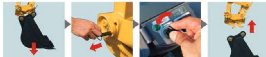
Place the bucket on the ground Pull out the safety lock pin Turn the switch to dismounting. Raise the arm to detach.
