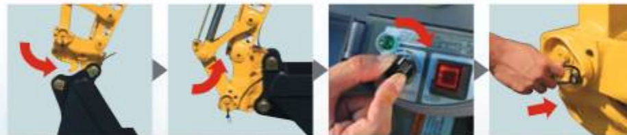
Apply the fixed hook Make the bucket level. Turn the switch to mounting Insert the safety lock pin and fasten.
